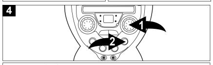
Adjust the MIC VOLUME control • as desired. Increasing this control will increase the volume of the microphone. Adjust the ECHO control • to add an echo effect to your voice. The ECHO control • is variable so add as much or as little reverb as desired. Sing or talk into the microphone and you will hear both the CD+G and the microphone.
